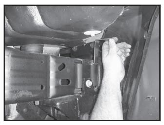
**6a.** Install bent nut strip through hole in frame and line up with rear hole used for tow hook. Install 1/2" x 2" bolt and 1/2" lock washer and tighten.
